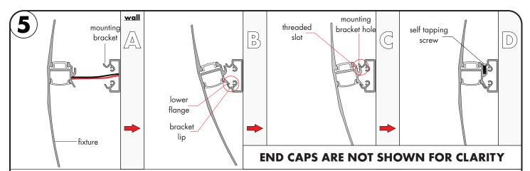
5.1 Insert the fixture lower flange into the mounting bracket lip. Then push the fixture threaded slot to the mounting bracket holes and secure using the provided self tapping screws, refer to diagram above for reference.
