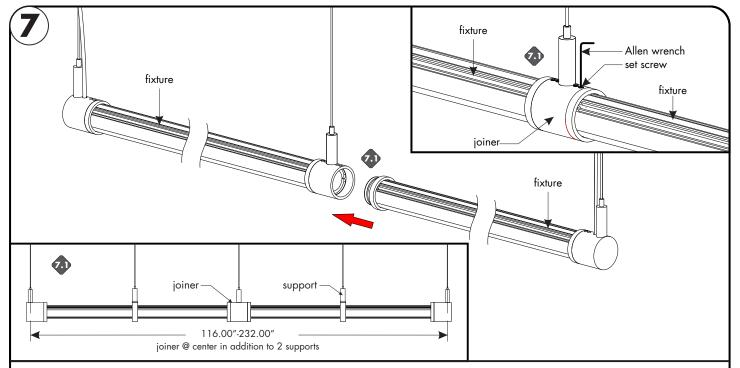
**7.1** If joining fixtures together, insert the fixture end into the corresponding fixture. Secure by tightening the two set screw that is the closest to the fixture. Reference drawing above as reference, to join correctly.
