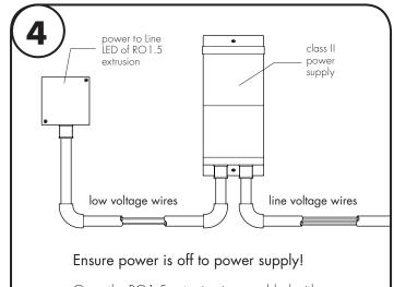
Once the RO1.5 extrusion is assembled with all parts and accessories, connect wires from Line LED to appropriate power supply. For more information please refer to power supply and Line LED wiring instructions.
