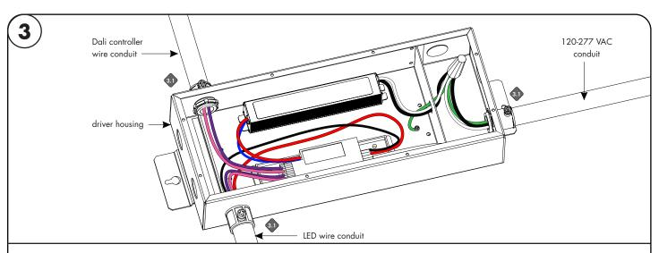
3.1 Insert the 120-277V AC power into the driver housing from the electrical panel. Followed by bringing 24V DC low voltage conduit one for the LED & other for controller wires. Refer to diagram on page 2 to make all the proper wiring connections.
