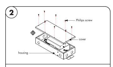
2.1 Remove the eight Phillips screws from the top of the driver housing and pull the cover off to expose the driver wires.
