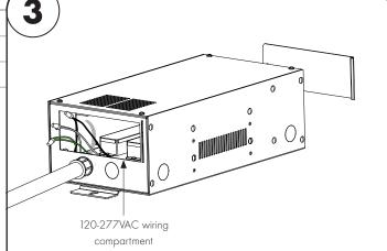
3.1 Connect the white (neutral) and black (hot) power supply wires to the white and black power wires ( 120 - 277 VAC ). Followed by connecting the ground wires in accordance with local electrical codes.
