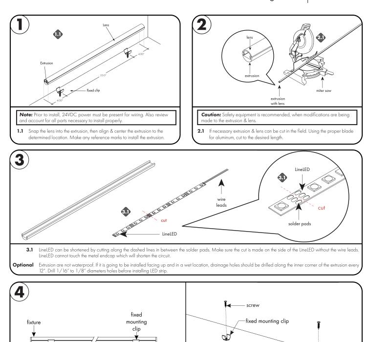
Align the mounting brackets to the edge of the surface, followed by securing each mounting bracket with 1 screw. Mounting bracket must be installed every 23". Snap
