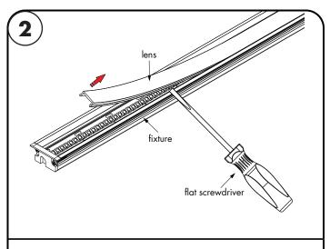
**2.1** Use a flat screwdriver to remove the fixture lens.
