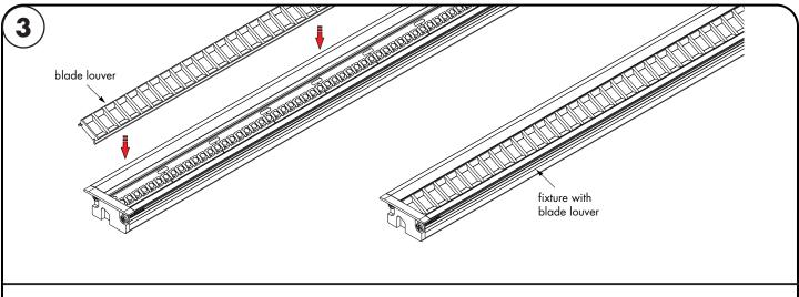
3.1 Snap the blade louver onto fixture.
