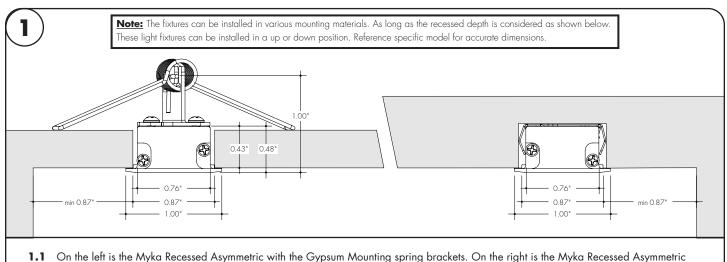
On the left is the Myka Recessed Asymmetric with the Gypsum Mounting spring brackets. On the right is the Myka Recessed Asymmetric with the Hard Surface Mounting brackets.
