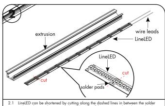
pads. Make sure the cut is made on the side of the LineLED without the wire leads. LineLED cannot touch the metal endcap which will shorten the circuit
