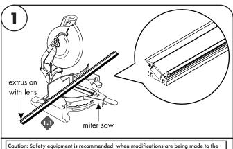
If necessary extrusion & lens can be cut in the field. Using the proper blade for aluminum, cut to the desired length.
