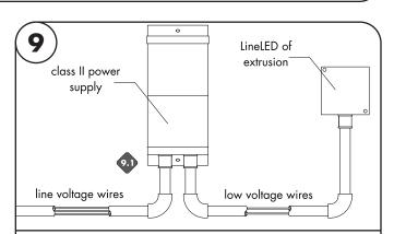
Ensure the correct (wattage & voltage) power supply is used to power LineLED. Then proceed to connect LineLED wires from extrusion to power supply. For more information please refer to power supply and LineLED wiring instructions.
