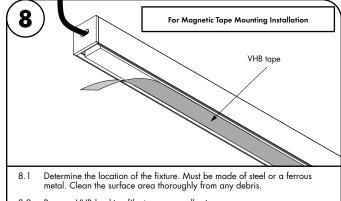
8.2 Remove VHB backing film to expose adhesive.
