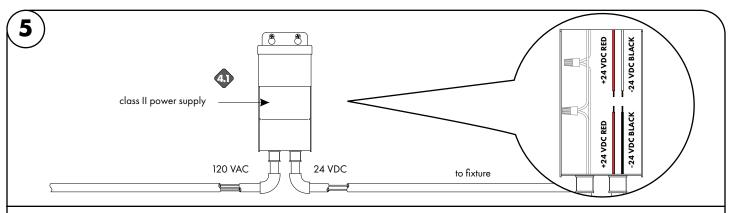
Connect +24 VDC red wire from the fixture to the power supplies +24 VDC red wire using a wire nut. Then connect the -24 VDC black wire from the fixture to the power supplies -24 VDC black wire using a wire nut.
