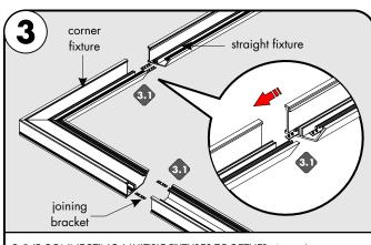
3.1 IF CONNECTING MULTIPLE FIXTURES TOGETHER: Insert the joining brackets into one of the fixture end(s) & tighten the screws on the bracket. Then slide the connecting fixture into the brackets and secure by tightening the screws on bracket.
