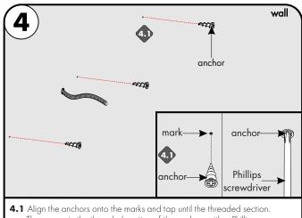
Then screw in the threaded portion of the anchors with a Phillips screw driver.
