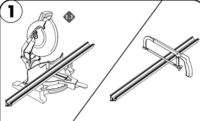
**1.1** If necessary cut the extrusion, reflector & cover to the desired length, with the proper equipment/tool that is appropriate to cut aluminum.
