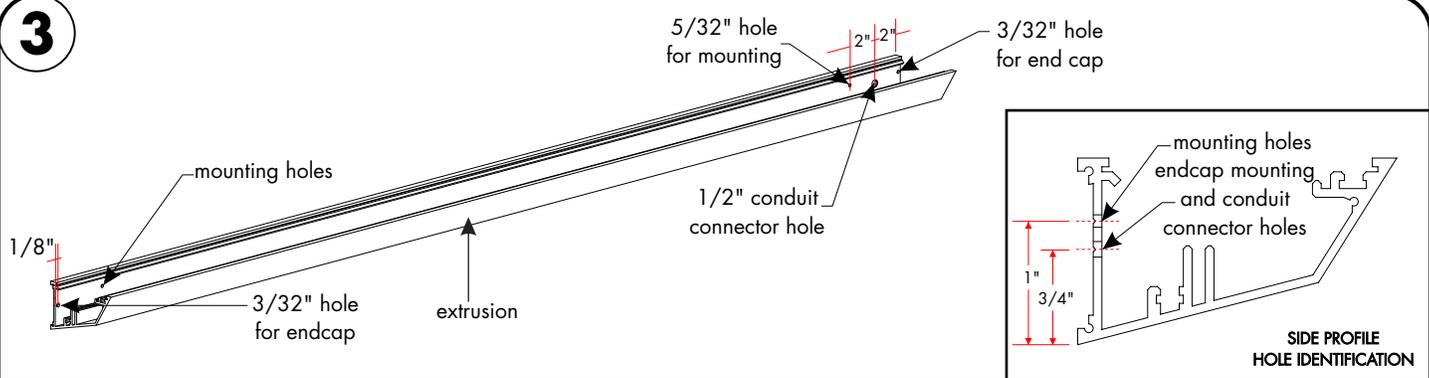
**3.1** Prior to installing the fixture, 3 sets of holes need to be made into the extrusion. Refer to drawing above to make all necessary holes to the extrusion. For installation to work properly.
