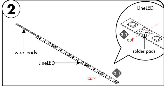
**2.1** LineLED can be shortened by cutting along the dashed lines in between the solder pads. Make sure the cut is made on the side of the LineLED without the wire leads. LineLED cannot touch the metal endcap which will shorten the circuit.
