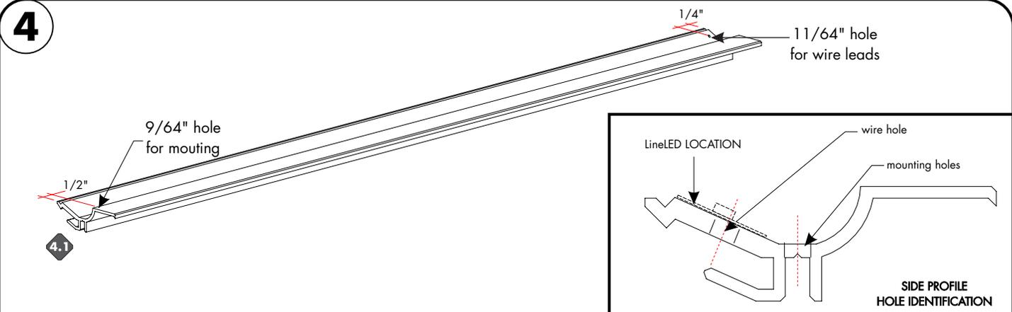
**4.1** Holes will also have to be made to the reflector, Refer to drawing above to make all necessary holes to the reflector.
