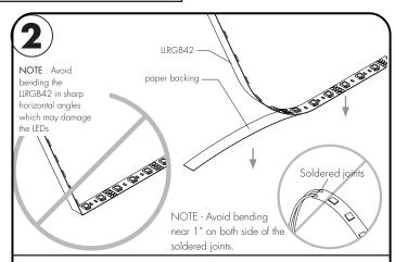
Remove the paper backing from the LLRGB42 and firmly press down making sure there are no air bubbles that can cause surface irregularities. Do not remove the adhesive, removing the adhesive may cause arcing of the Line LED tape.
