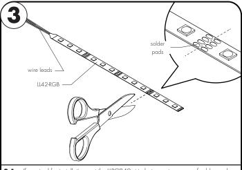
If required for installation, cut the LLRGB42 strip between two rows of solder pads. Always cut LLRGB42 from end without connector / wire leads.
