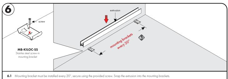
6.2 To remove the extrusion from the mounting brackets, carefully insert a flat screwdriver to the bottom edge of the extrusion then pull up until the extrusion pops up.
