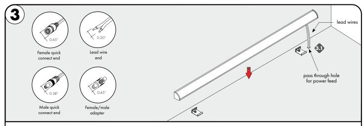
3.1 If necessary make any pass through holes for wire lead/connector to the surface, depending on the power feed option. Then snap the fixture into the fixed mounting clip to secure in place. Diagram on the right side illustrates the common way of connecting multiple fixtures to each other, depending on the location of the power feed wires.
