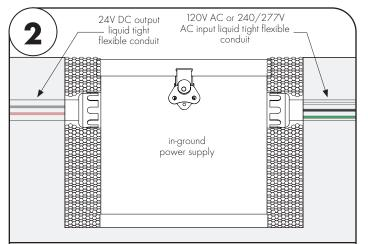
Install as shown, routing wiring through liquid tight conduit and conduit connectors. Once installed, care must be taken to ensure the enclosure remains watertight, keeping top cover seal free of debris. Secure cover by rotating both wing latches fully clockwise. There are two 3/4" conduit openings provided in the enclosure, shipped from the factory with seal-tight plugs installed. Any unused plugs must remain in place.
