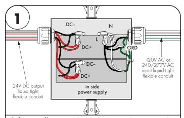
**Before installing,** check the label and ensure the power supply has the proper input voltage, output voltage, and wattage for the job. Check the wire markings to ensure they match the wiring diagram below. Refer to table above for the maximum loads supported by each power supply.
