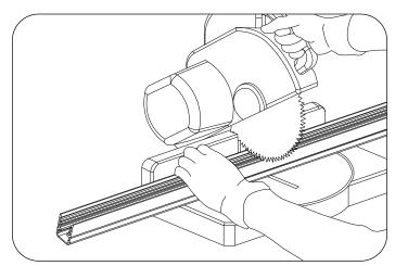
2 Take reduced measurements and cut cap rail housing to length with chop saw. If using lens, cut lens to same length as cap rail housing. Do not cut both at same time.
