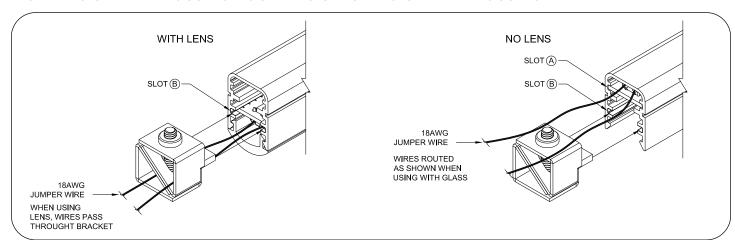
7 If using lens, feed 18 AWG jumper wire through LED mounting clip as shown (above left), and slide clip in cap rail into Slot B.
