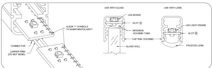
3 Slide LED light engine boards into cap rail housing slot. If using with glass, place LED light engine board into slot (A). Slot options (A) or (B) are available if using with lens. Once inserted, take two jumper pins and insert into female connectors on end of LED light engine board light. To connect LED boards, align the "+++" of the first board to the "+++" on the second LED board. Press the two tabs on the connector to remove jumper pins and lead wires.
