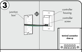
3.1 Loosen the screws on the back of the controller housing and make all the proper wiring and then re-tighten screws. Refer to the wiring diagram on page 2 for additional information.
