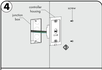
4.1 Align the controller housing to the junction box and secure using the two screws.
