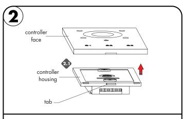
2.1 Carefully insert a flat screw driver into the controller housing tab and slightly pull up until controller face comes off.
