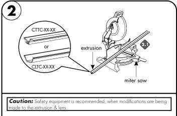
2.1 If necessary extrusion can be cut in the field, using the proper blade for aluminum. Cut the extrusion to the desired length.
