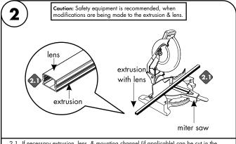
If necessary extrusion, lens, & mounting channel (if applicable) can be cut in the field. Snap all parts together then using the proper blade for aluminum cut to the desired length.
