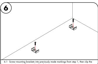
extrusion on to the mounting brackets.
