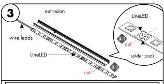
Note: Extrusion are not waterproof. If it is going to be installed facing up and in a wet location, drainage holes should be drilled along the inner corner of the extrusion every 12". Drill 1/16" to 1/8" diameters holes before installing LED strip
