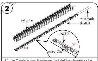
2.1 LineLED can be shortened by cutting along the dashed lines in between the solder pads. Make sure the cut is made on the side of the LineLED without the wire leads. LineLED cannot touch the metal endcap which will shorten the circuit
