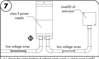
6.1 Ensure the correct (wattage & voltage) power supply is used to power LineLED. Then proceed to connect LineLED wires from extrusion to power supply. For more information please refer to power supply and LineLED wiring instructions.
