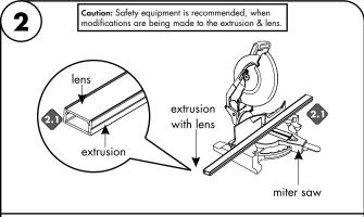
2.1 If necessary extrusion, lens, & mounting channel (if applicable) can be cut in the field. Snap all parts together then using the proper blade for aluminum cut to the desired length.
