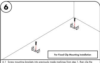
6.1 Screw mounting brackets into previously made markings from step 1, then clip the extrusion on to the mounting brackets.
