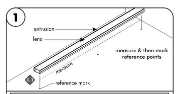
Note: Complete fixture must be built prior to installing. To make all necessary reference marks & to also ensure all parts are included. Then it can be taken apart for installation.
