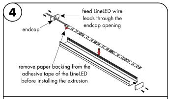
4.1 Prior to installing LineLED to extrusion, clean extrusion from any debris. Gently push LineLED onto aluminum extrusion. Then install endcaps at each ends of the extrusion.
