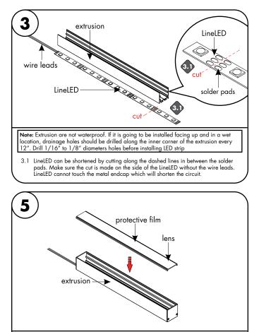
5.1 Remove the protective film from the diffuser lens. Snap the diffuser lens into the aluminum extrusion.
