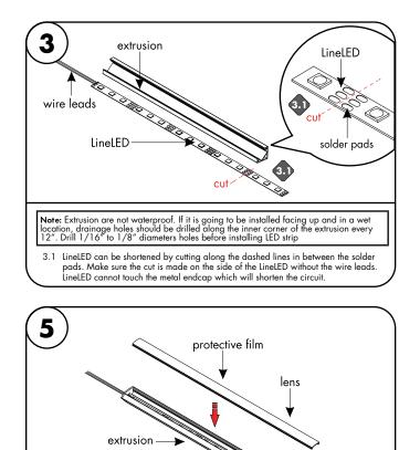
5.1 Remove the protective film from the diffuser lens. Snap the diffuser lens into the
