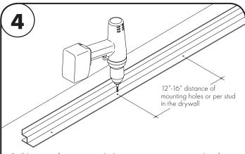
Drill location for mounting holes at appropriate intervals, after locating stud supports in the wall. Ensure appropriate drill bit is used to drill in the aluminum extrusion.
