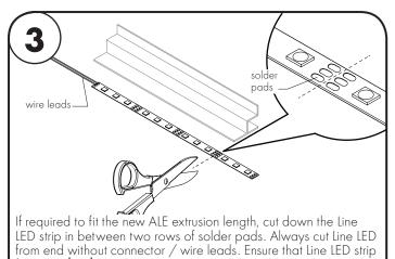
fits completely inside the extrusion and the solder pads do not
