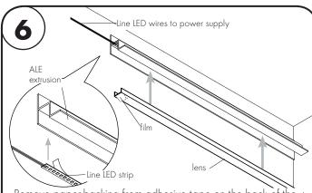
Remove paper-backing from adhesive tape on the back of the 1 Line LED strip before installing onto the ALE extrusion. Once the Line LED strip is in place, snap on the diffuser lens. Remove the protective film from the lens.
