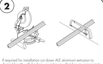
If required for installation cut down ALE aluminum extrusion to desired length with hacksaw or miter saw that has an appropriate blade for cutting aluminum. Always wear safety goggles when cutting.
