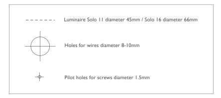
**NOTE** Model shown is the Solo 16 LED. The same procedures apply for Solo 11 LED.
