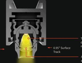
Titanium-dioxide, Chip-Scale Package (CSP) LEDs direct all light forward, enabling the use of a singular micro-optic for each LED
