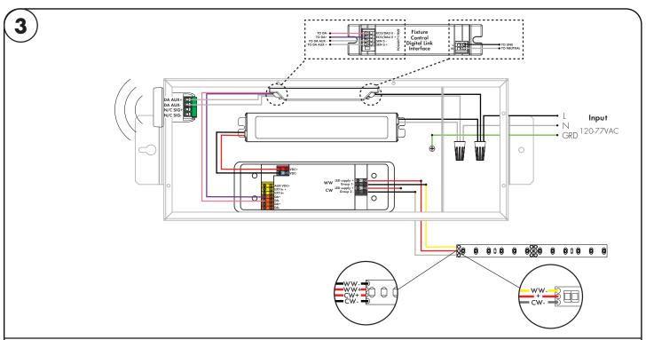
3.1 Insert the 120-277V AC power into the driver housing from the electrical panel. Followed by bringing 24V DC low voltage conduit one for the LED & other for controller wires.
