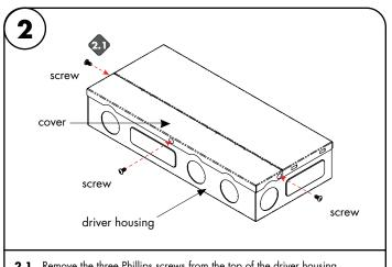
Remove the three Phillips screws from the top of the driver housing 2.1 and pull the cover off to expose the driver wires.
