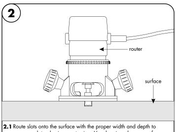
accommodate aluminum extrusion. Use drawing above as reference.
