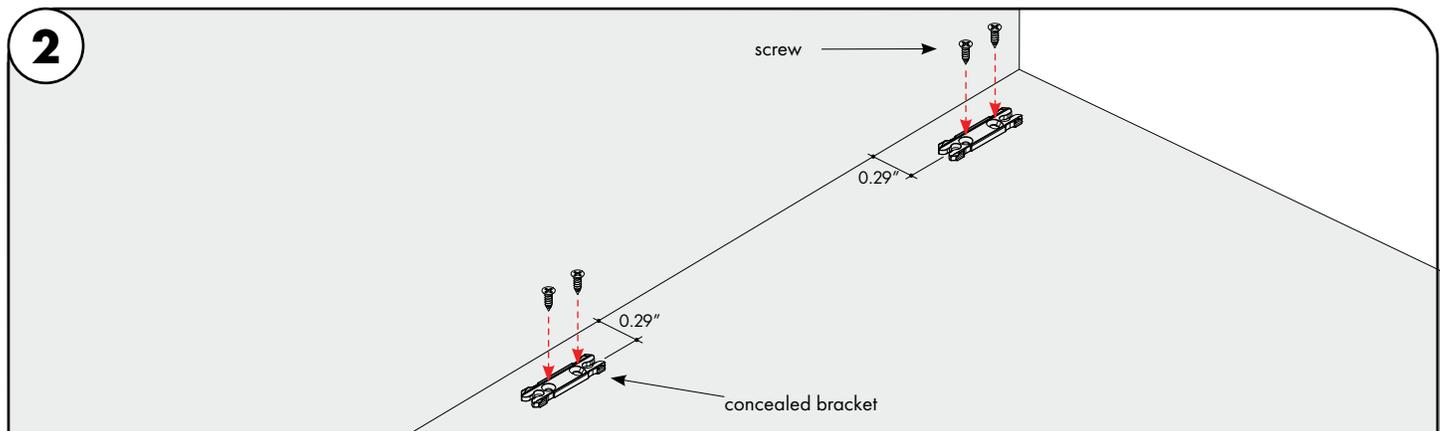
**2.1** Align the mounting brackets to the marks, followed by securing each mounting bracket with 2 screws. Snap the extrusion into the mounting brackets.
