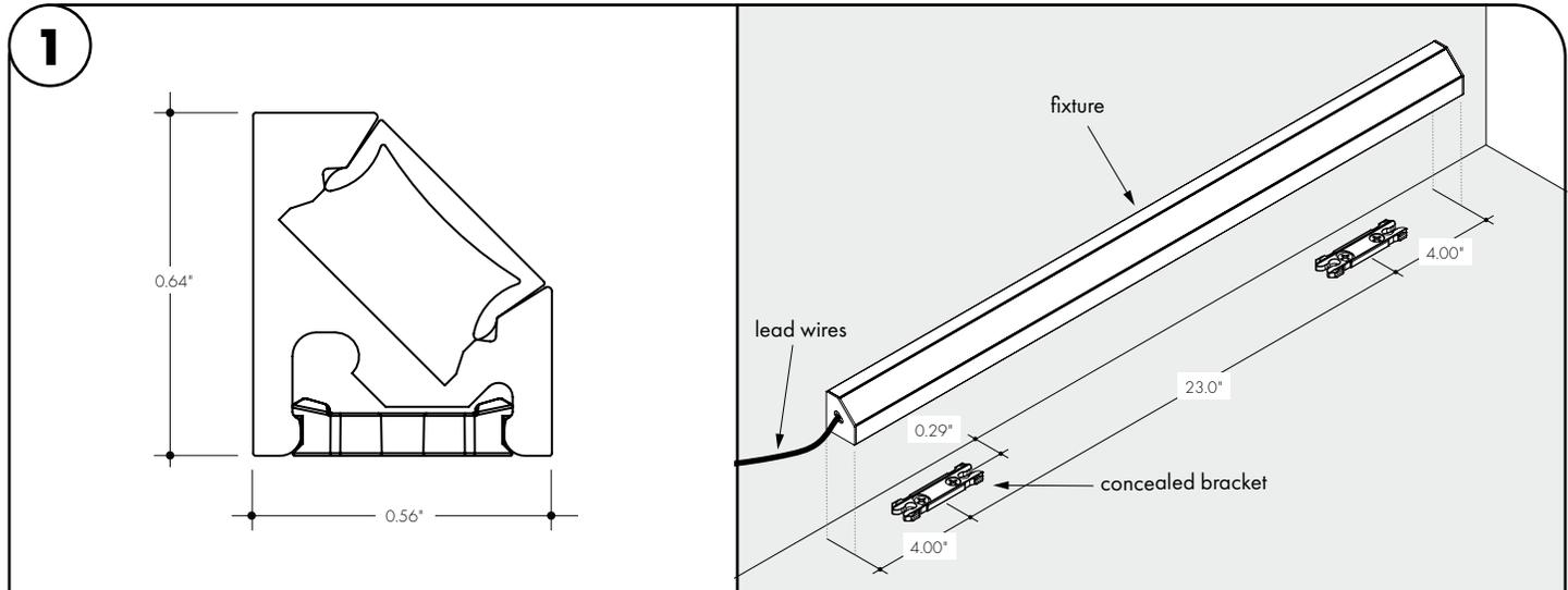
**1.1** Determine the location of where the fixture(s) will be installed. Lay the fixture(s) on the surface, and make any necessary reference marks for the concealed bracket. Make marks 4" from each end of the fixture(s) and also every 23" in between. Use the fixture profile and mounting bracket detail, for any additional details.
