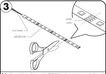
If required for installation, cut the LLRGBW36 strip between two rows of solder pads.
