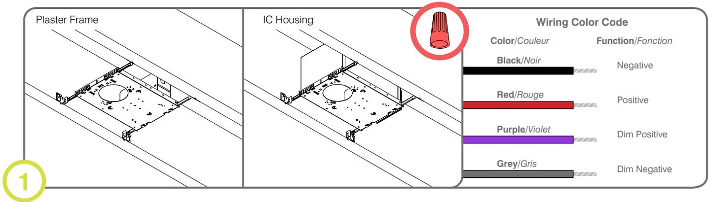
Install appropriate housing between ceiling joists. Connect the driver to the line voltage and ground to enclosure.
