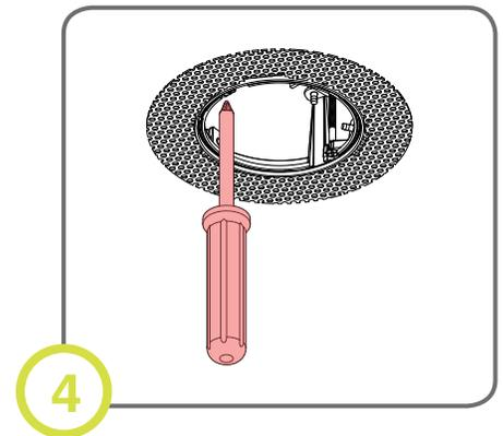
Turn screws to secure fixture to ceiling.
