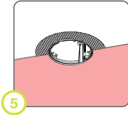
Mud over area between fixture and ceiling. Wipe any excess inside trim.
