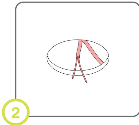
Finish ceiling installation. Make sure hole is cut to appropriate size and location.
