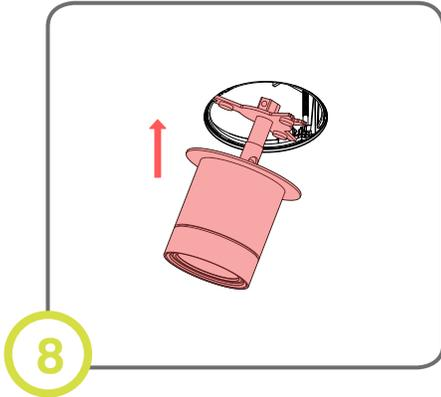
Rest the three arm ends in the notches in the trim. Push the trim plate back against the arms.
