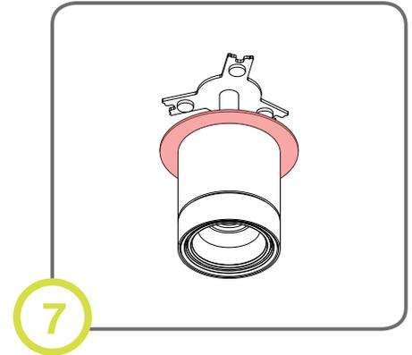
Separate trim plate from bracket and insert the fixture into the ceiling.
