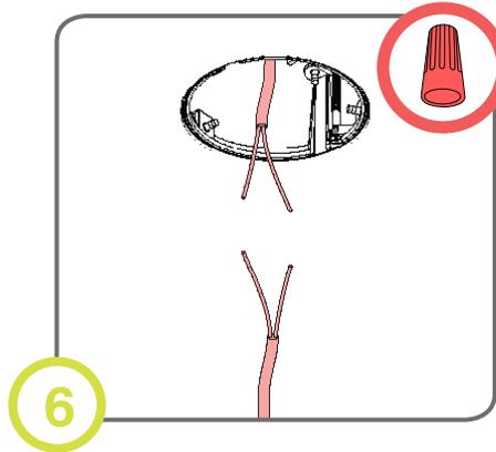
Ensure power is off and make electrical connections.
