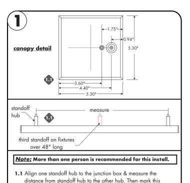
location to the ceiling. Make addition marks if using more than one standoffs. Use canopy detail to slighting off center standoff
