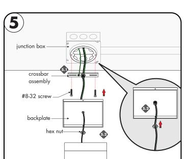
**5.1** Align the crossbar to the junction box holes and secure using the provided two #8-32 screw.
