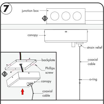
7.1 Insert the low voltage wire nut connections into the canopy. Align the canopy to the backplate and securing using the 4 Phillip screws.
