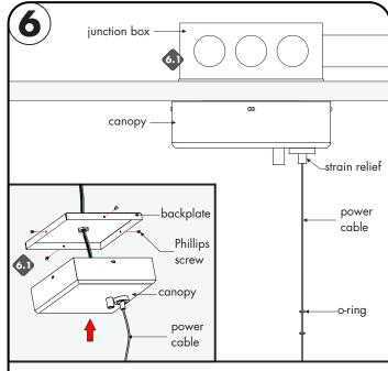
**6.1** Insert the low voltage wire nut connections into the canopy. Align the canopy to the backplate and securing using the 4 Phillip screws.
