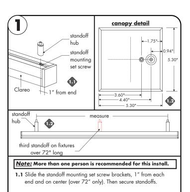
1.2 Determine length from the canopy to the standoff hub. Then mark this location to the ceiling. Make addition marks if using more than one standoffs. Use canopy detail to slighting off
