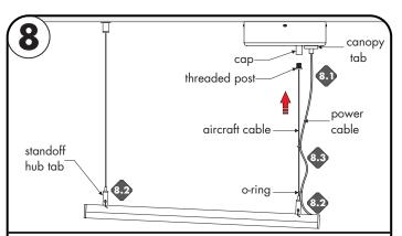
Align the canopy to the backplate and securing using the 4
