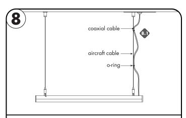
8.1 If necessary make any final adjustments to the cables use the o-rings for a cleaner look.
