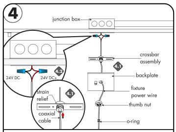
Note: Prior to wiring the desired fixture height must be determined to cut off any un-necessary wire.
