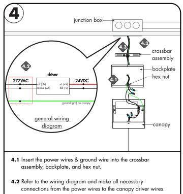
4.3 Connect to ground in accordance with local electrical codes.
